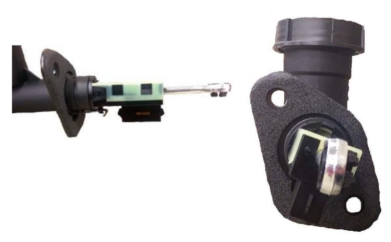
**Note: Installation orientation of clip/switch is critical!**
