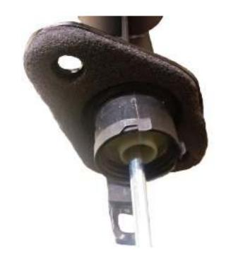
8. Slide clip down into the groove of the new master cylinder making sure that the clip ends lock in behind the location tabs as shown in step 1.
