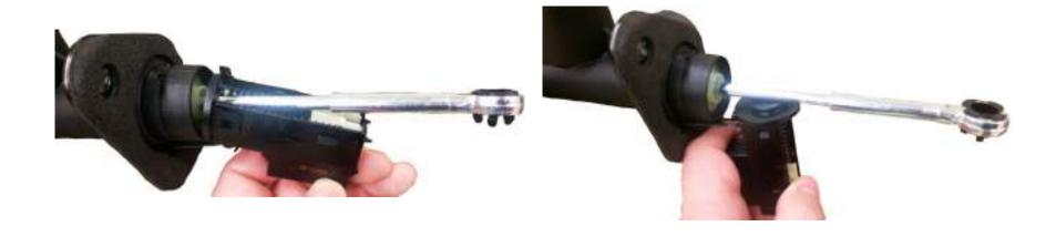
4. Take note how clip ends are locked in behind the position tabs on the master cylinder housing. Will need to make sure that the clip ends are in the same position when the clip is assembled to the new
