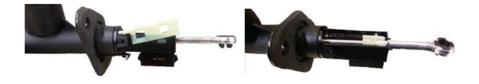
3. To remove the switch, push down on the switch un-clipping it from the pushrod. Continue pulling down on the switch to remove the location tab from the retention clip.
