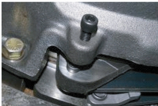
Broken ear with jackscrew in place
