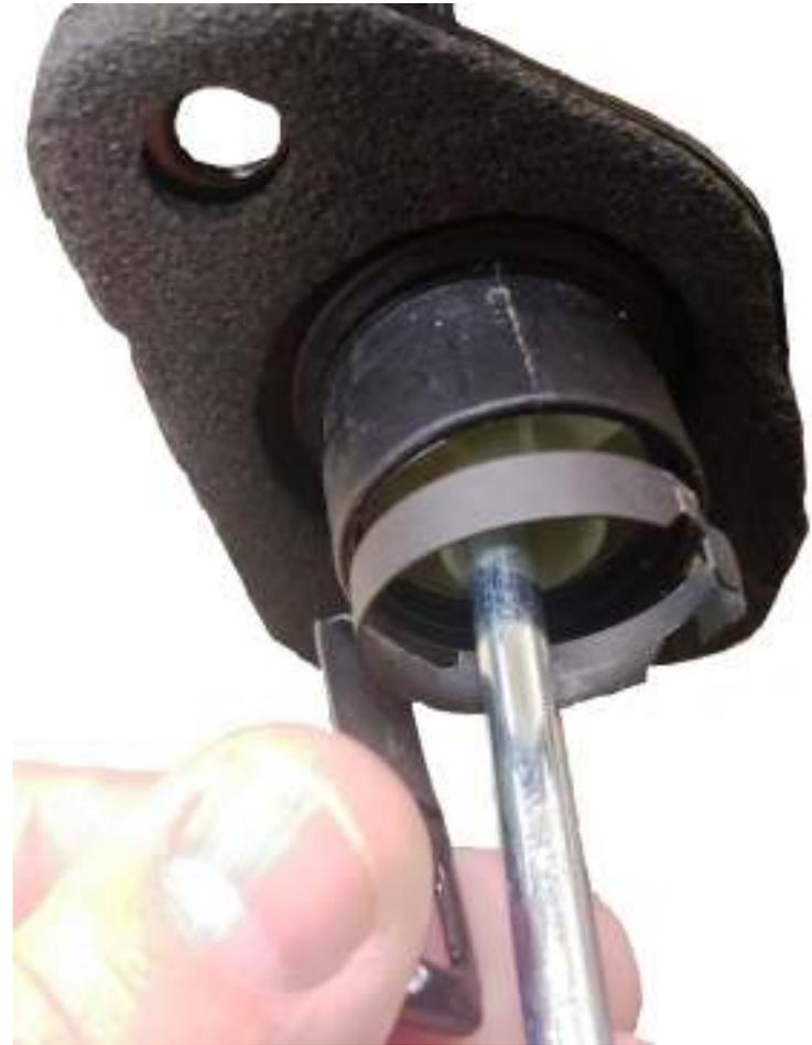
**7. Spread the ends of the clip apart and slide over the bore end of the new master cylinder.**
