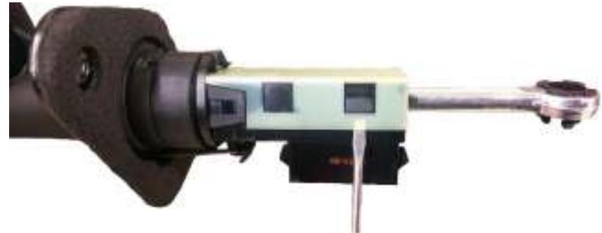
**2. Lift switch cover up and remove from the switch.**
