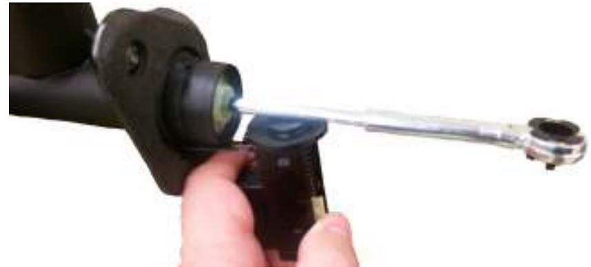
**4. Take note how clip ends are locked in behind the position tabs on the master cylinder housing. Will need to make sure that the clip ends are in the same position when the clip is assembled to the new master cylinder housing.**
