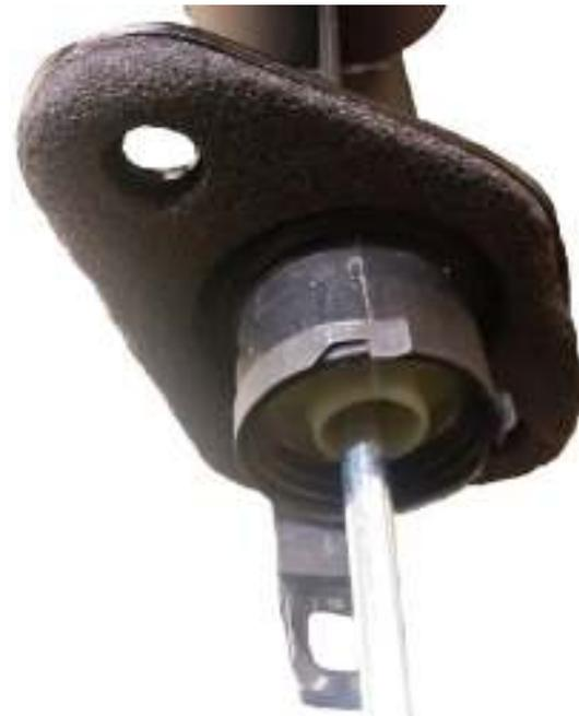
**8. Slide clip down into the groove of the new master cylinder making sure that the clip ends lock in behind the location tabs as shown in step 1.**
