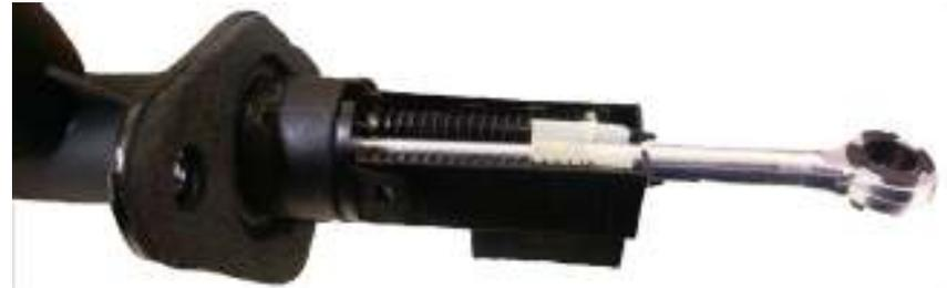
**3. To remove the switch, push down on the switch un-clipping it from the pushrod. Continue pulling down on the switch to remove the location tab from the retention clip.**
