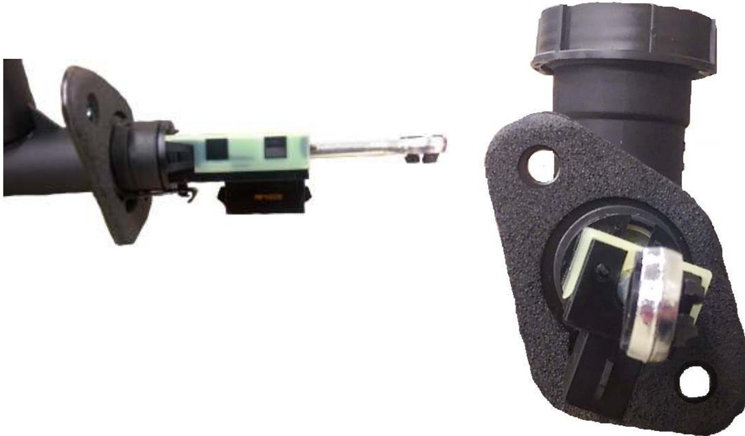
**Note: Installation orientation of clip/switch is critical!**
