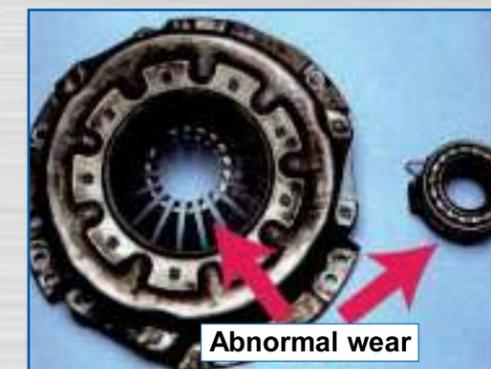
2) Excessive wear on diaphragm tips
