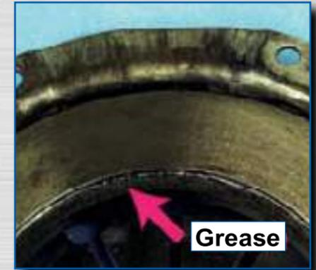
Grease on friction surface
