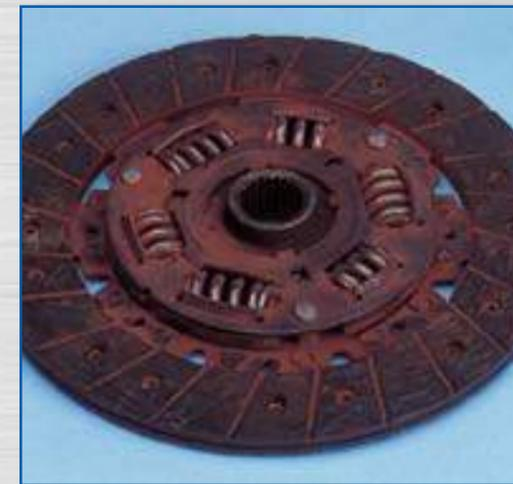
**PROBLEM:** Torque stopper springs broken. Difficult gear engagement which may lead to clutch failure.
