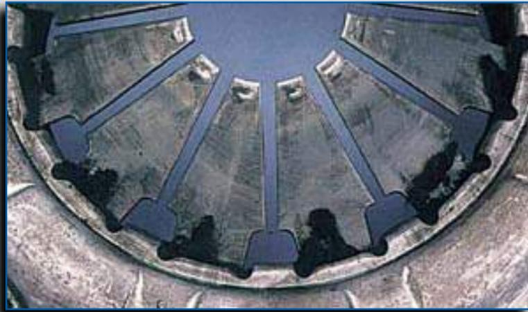
**PROBLEM:** Worn clutch disc facing fibres and dirt lodged between diaphragm spring and clutch cover housing causing loss of clamp load.
