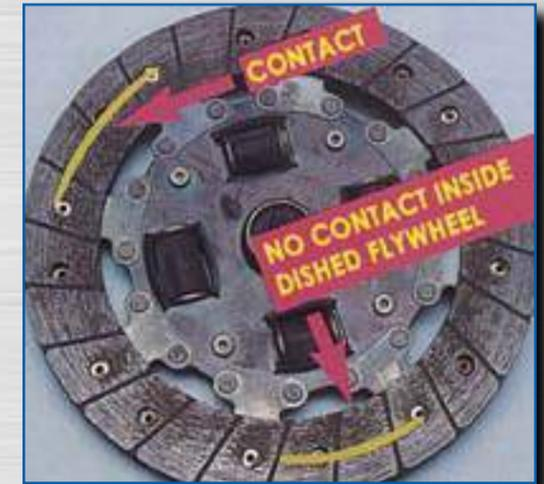
**PROBLEM:** Highly glazed to a mirror finish pressure plate cover assembly casting/red dust on clutch components.
