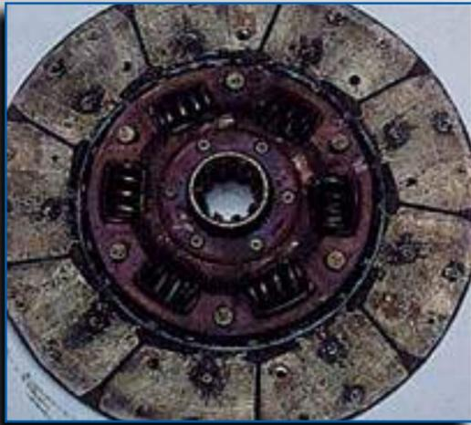
**PROBLEM:** Different number of spline on main drive to those on clutch disc/diameter of spline incorrect.
