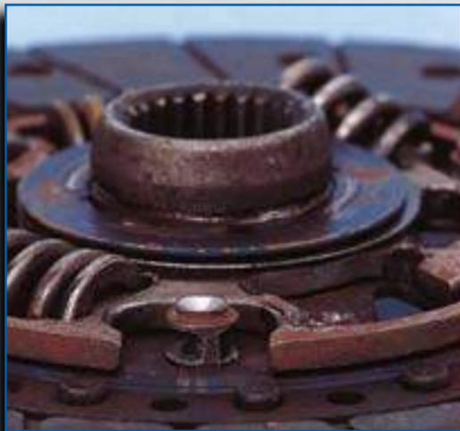
**PROBLEM:** Torsion dampener stopper springs thrown out of side plate/stop pins worn.
