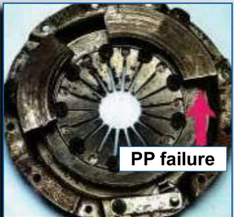
Breakage of pressure plate
