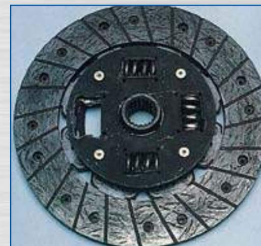
**PROBLEM:** Wrong type of lubrication on input shaft spline.
