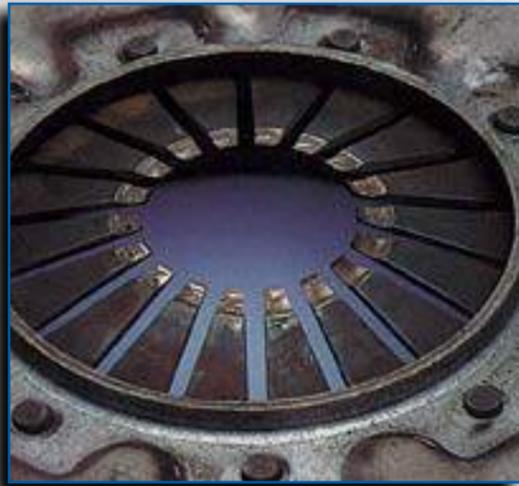
**PROBLEM:** Excessive wear on diaphragm tips and a highly glazed pressure plate casting.
