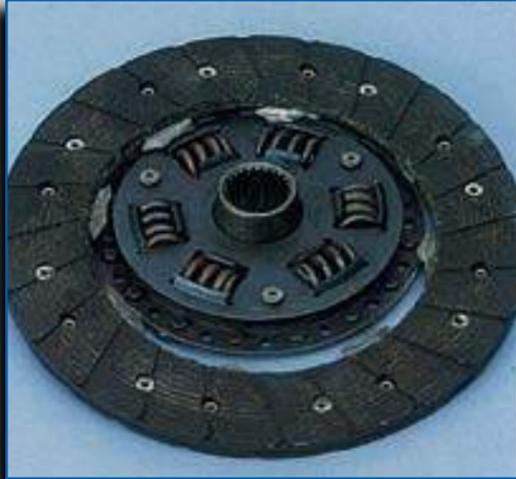
**PROBLEM:** No drive, power not transmitted because of broken segments on clutch disc.
