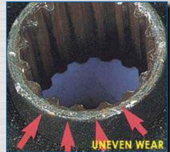
**PROBLEM:** Noisy and cannot transfer power/splines completely disintegrated.
