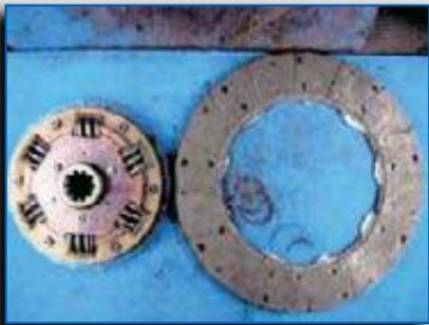
Separated clutch disc assembly
